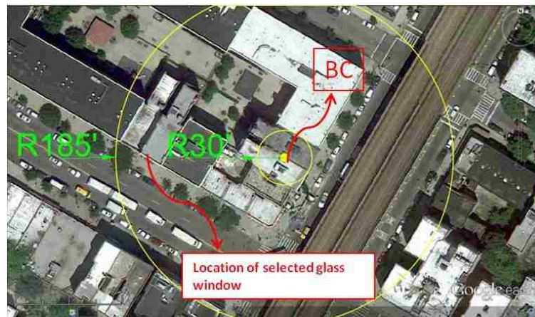
Figure 38 Blast center (BC) and selected glass window locations
