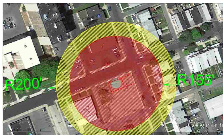
Figure 47 Growing area of windows damage for Allentown accident (Pso=0.3 psi)
