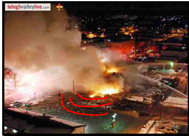
Figure 19 Fragments distribution around the demolished house [5].
